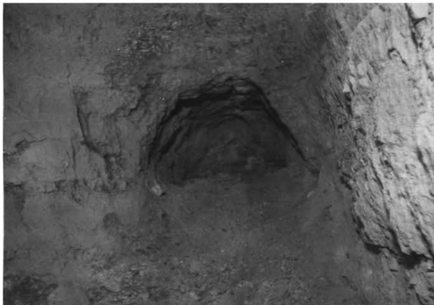
Photograph 14B. Results of Burn Cut Number 14 Visible Depth of Cut is 8 feet.
