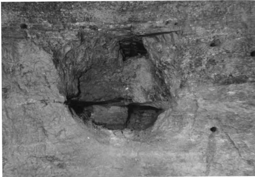
Photograph 6. Results of Burn Cut Number 6
