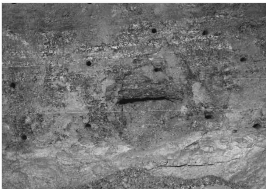
Photograph 10B. Results of Burn Cut Number 10 After Repriming and Shooting Holes 0, 1, and 2.
