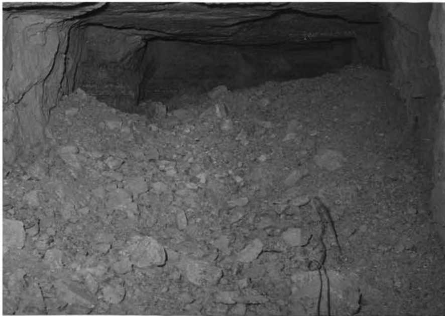
Photograph 8B. Muck Pile For Round 8. Fragmentation of Round Was Typical of All Test Rounds.
