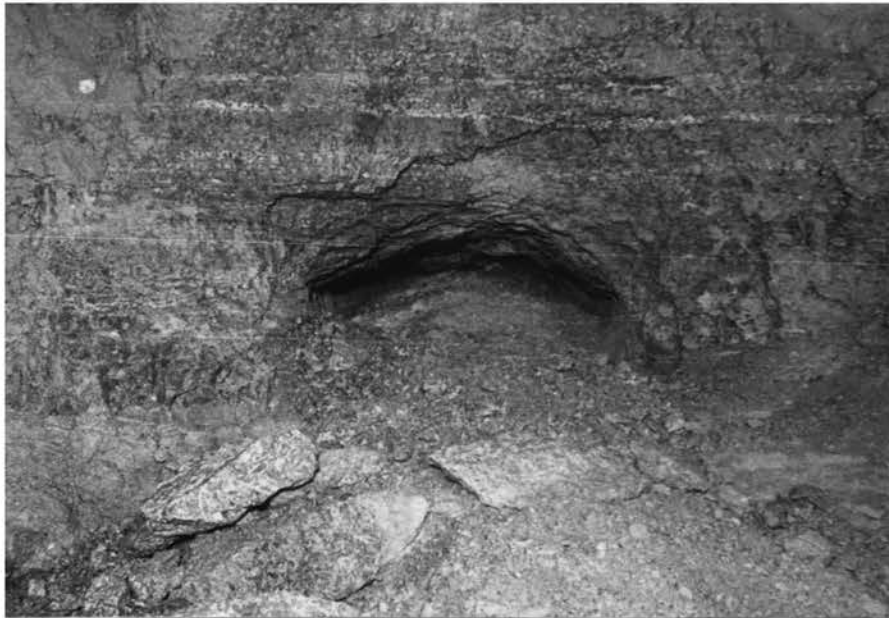
Photograph 8A. Results of Burn Cut Number 8. Bottom of Cut Visible in Picture is 9\frac{1}{2} Feet From Original Face.
